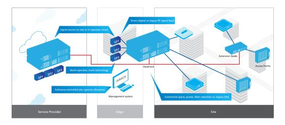
ERA's architecture scales from single buildings to large campuses and bases, while offering flexibility on the placement of system headend resources.
