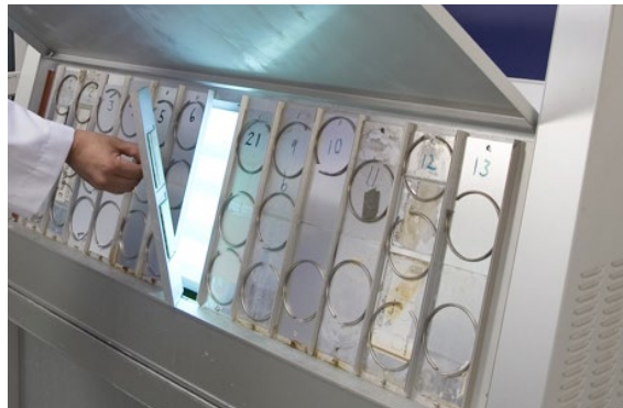
11.5: (Middle) and 11.6: (Right) UV aging test and continuous field exposure
