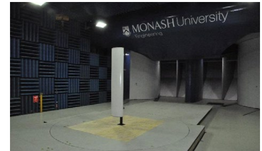
11.11: Wind tunnel testing of a base station antenna
